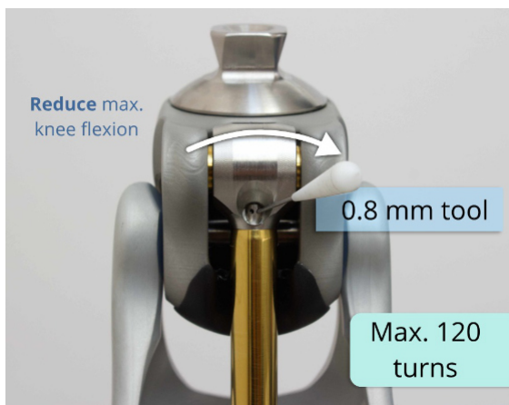
Fig 4.1: Adjustment of the maximum knee flexion
